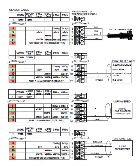
NOTE: To program the combination card analog input, you must go to Inputs menu, then enter the analog input (S13 or S23), scroll down to Transmitter, and select the type of transmitter from the list.
