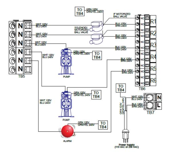
Figure 14 W600 AC Power & Relay Output Wiring
