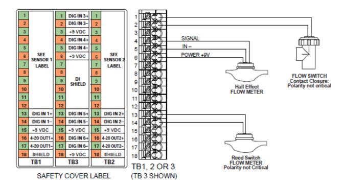
Figure 13 Digital Input Wiring
