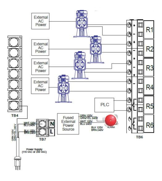
Figure 17 W640 AC Power & Relay Output Wiring
