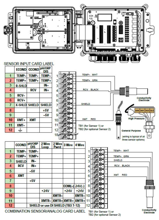
Figure 7 Contacting Conductivity Sensor Input Wiring
