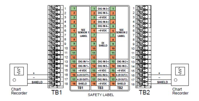
Figure 18 Analog Output Wiring
