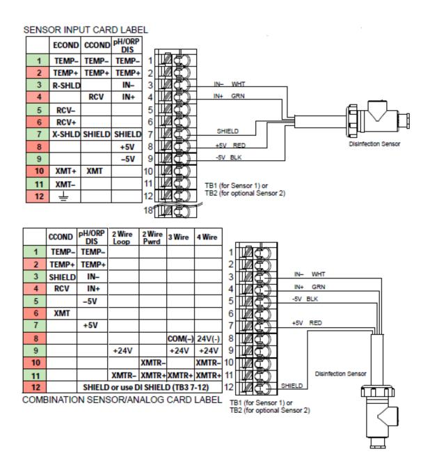
Figure 10 Disinfection Sensor Input Wiring
